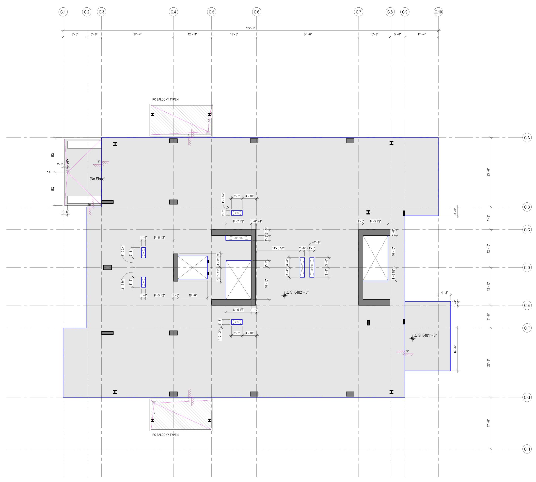
1 CONCRETE PLAN - TOWER C - LVL 3 SCALE: 1/8" = 1'-0"
