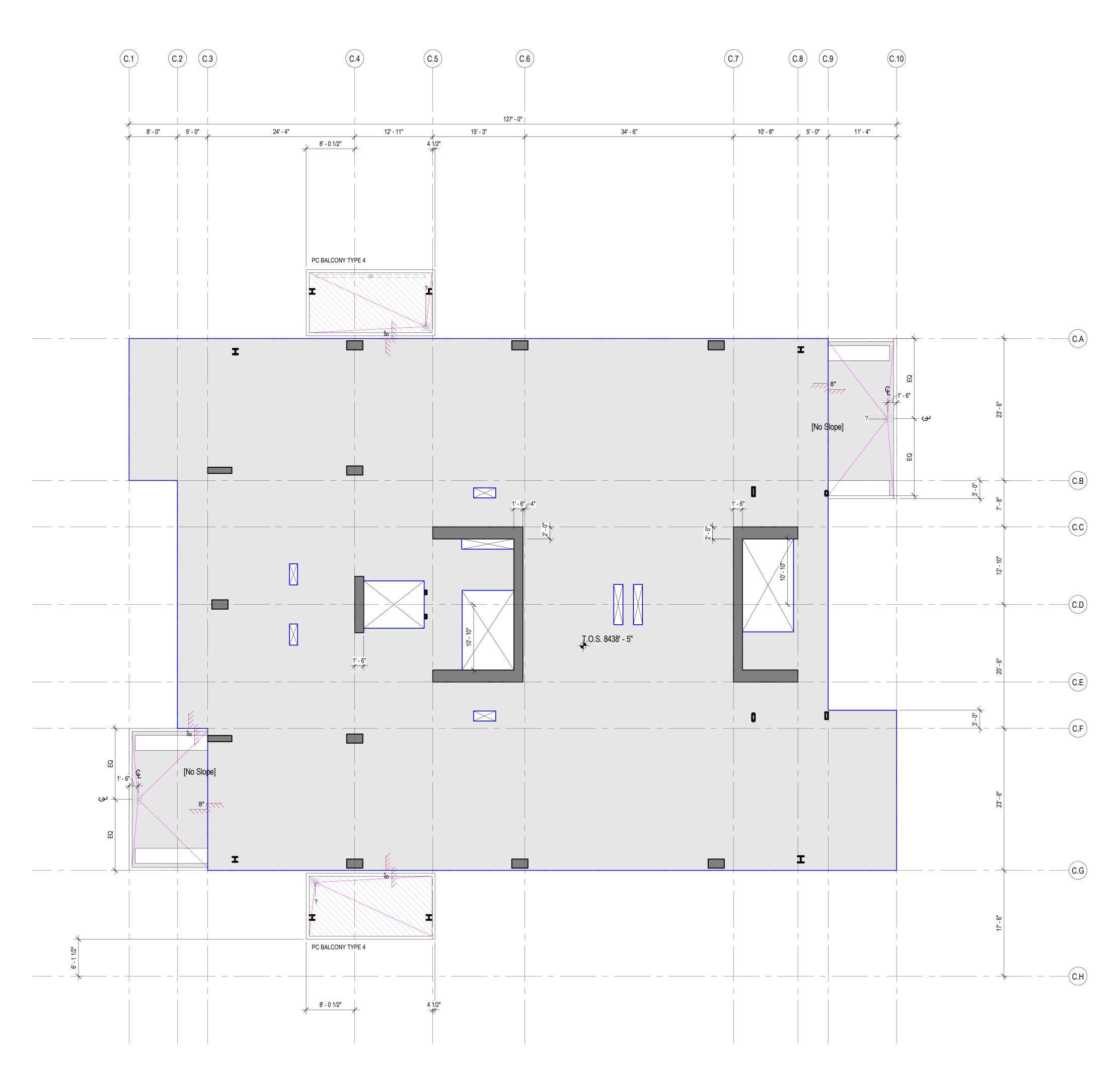
1 CONCRETE PLAN - TOWER C - LVL 6 SCALE: 1/8" = 1'-0"
