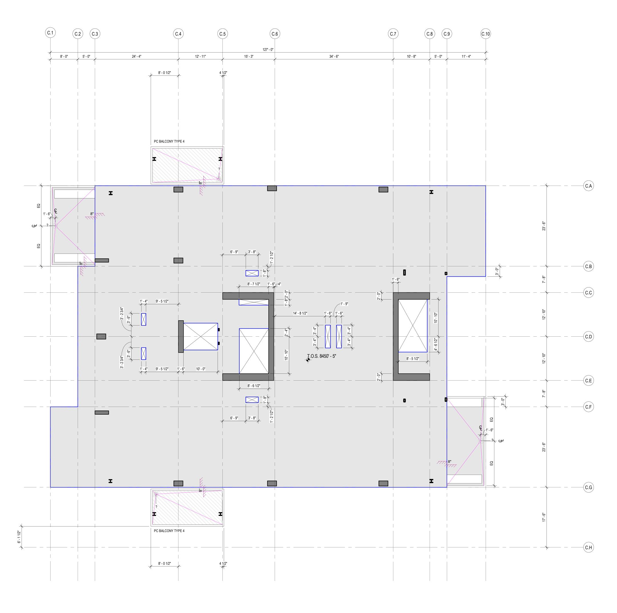
1 CONCRETE PLAN - TOWER C - LVL 7 SCALE: 1/8" = 1'-0"
