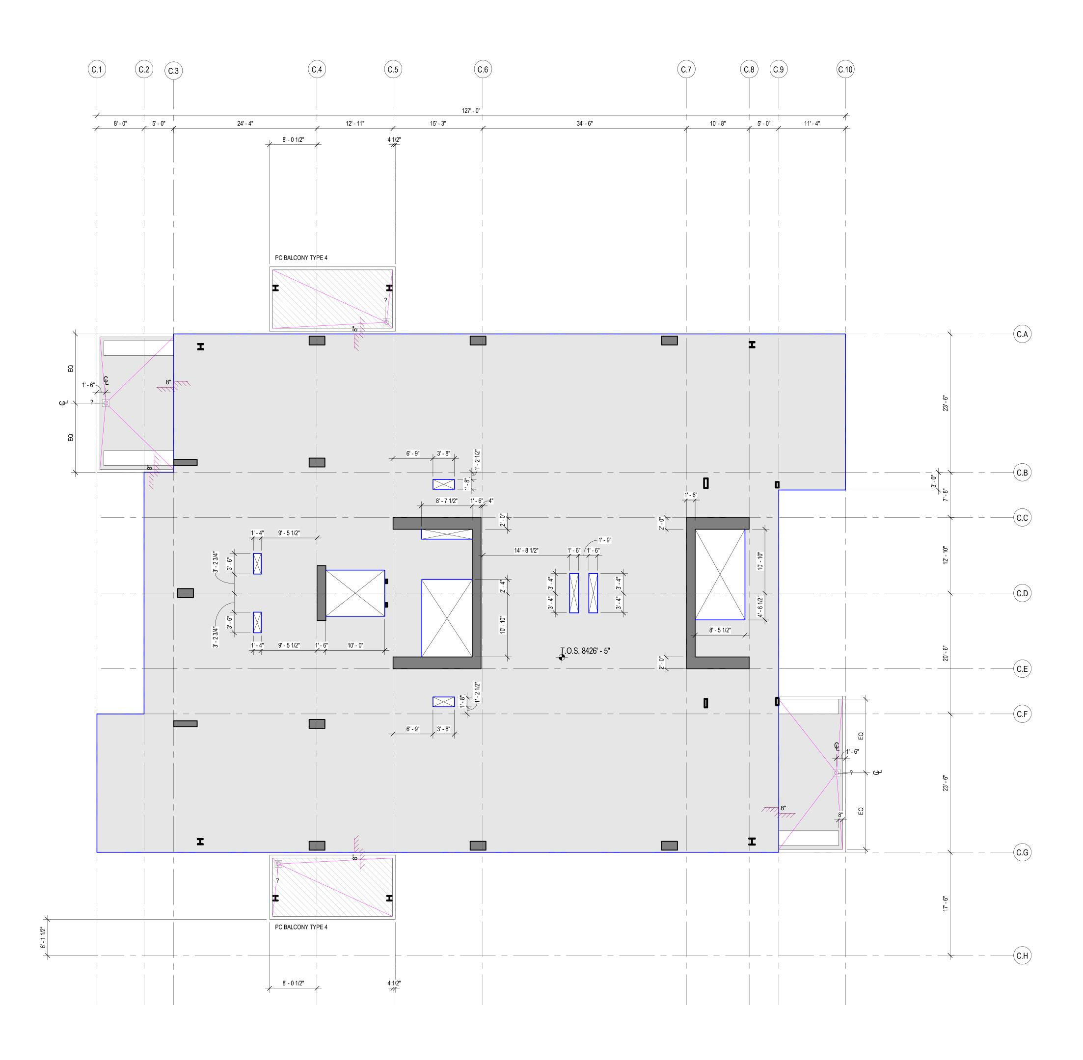
1 CONCRETE PLAN - TOWER C - LVL 5 SCALE: 1/8" = 1'-0"
