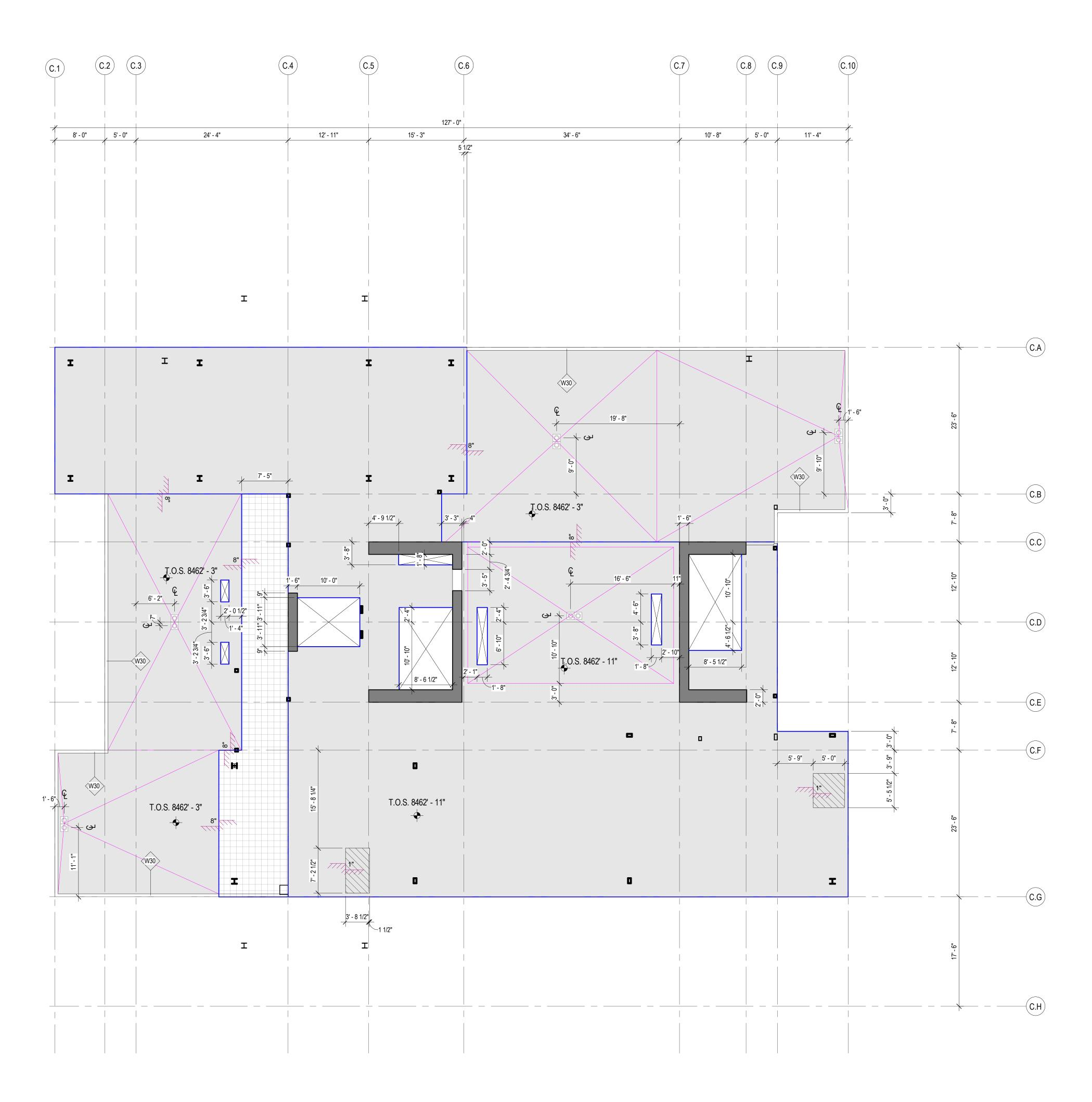
1 CONCRETE PLAN - TOWER C - LVL 8 SCALE: 1/8" = 1'-0"
