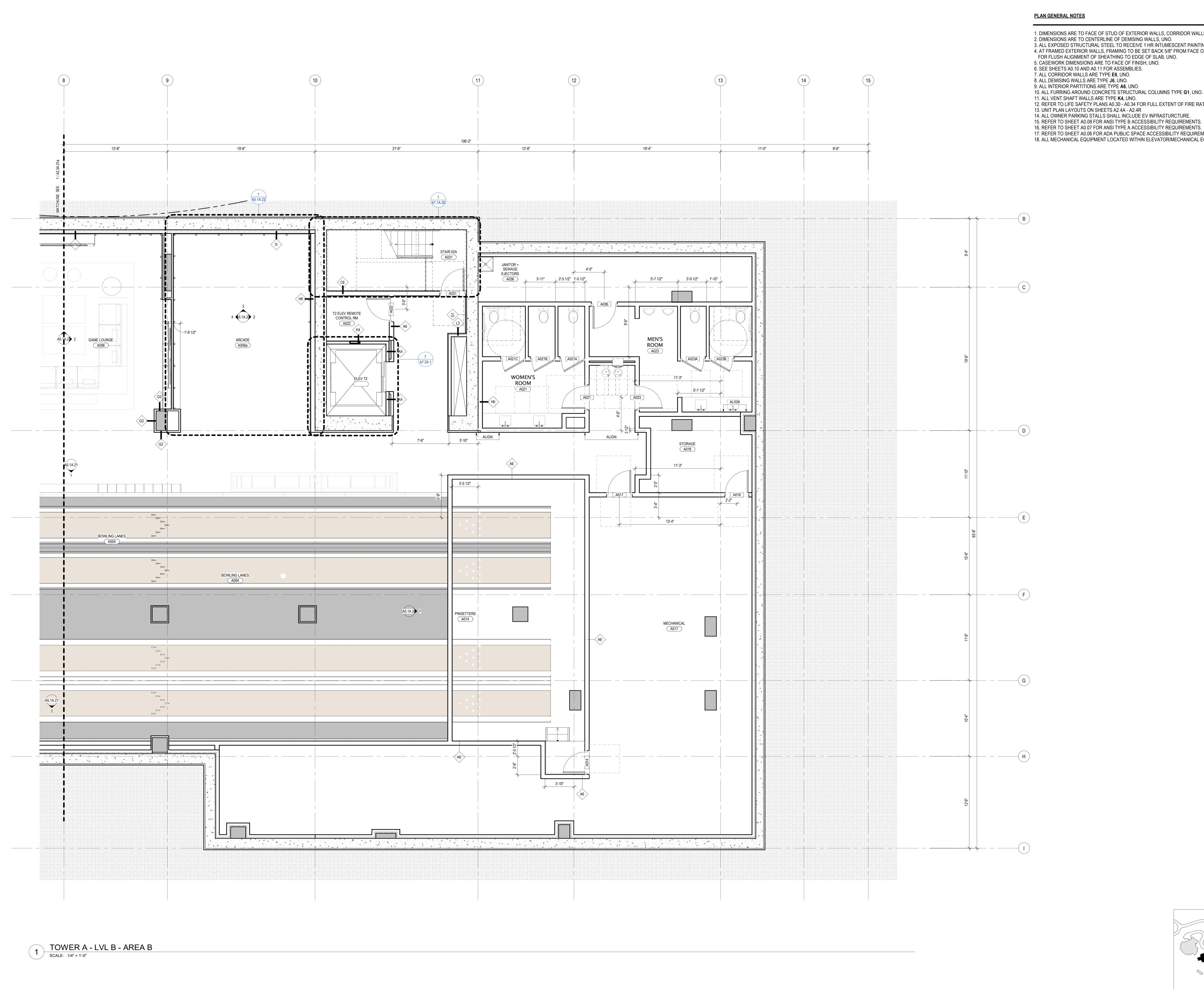
1. DIMENSIONS ARE TO FACE OF STUD OF EXTERIOR WALLS, CORRIDOR WALLS & INTERIOR WALLS, UNO 2. DIMENSIONS ARE TO CENTERLINE OF DEMISING WALLS, UNO. 3. ALL EXPOSED STRUCTURAL STEEL TO RECEIVE 1 HR INTUMESCENT PAINTING, UNO. 4. AT FRAMED EXTERIOR WALLS, FRAMING TO BE SET BACK 5/8" FROM FACE OF CONCRETE TO ALLOW FOR FLUSH ALIGNMENT OF SHEATHING TO EDGE OF SLAB, UNO.
