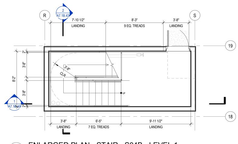
2 ENLARGED PLAN - STAIR - S04B - LEVEL 1 SCALE: 1/4" = 1'-0"
