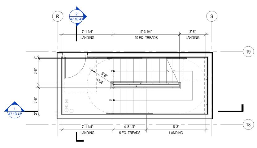
4 ENLARGED PLAN - STAIR - S04B - LEVEL 2 SCALE: 1/4" = 1'-0"
