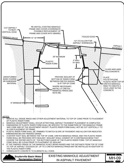
**EXISTING MANHOLE ADJUSTMENT IN ASPHALT PAVEMENT**
