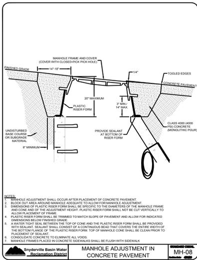
**MANHOLE ADJUSTMENT IN CONCRETE PAVEMENT**
