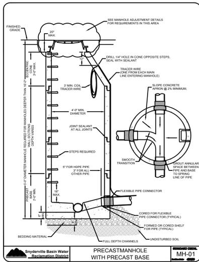
**PRECAST MANHOLE WITH PRECAST BASE**
