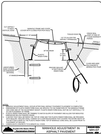
**MANHOLE ADJUSTMENT IN ASPHALT PAVEMENT**
