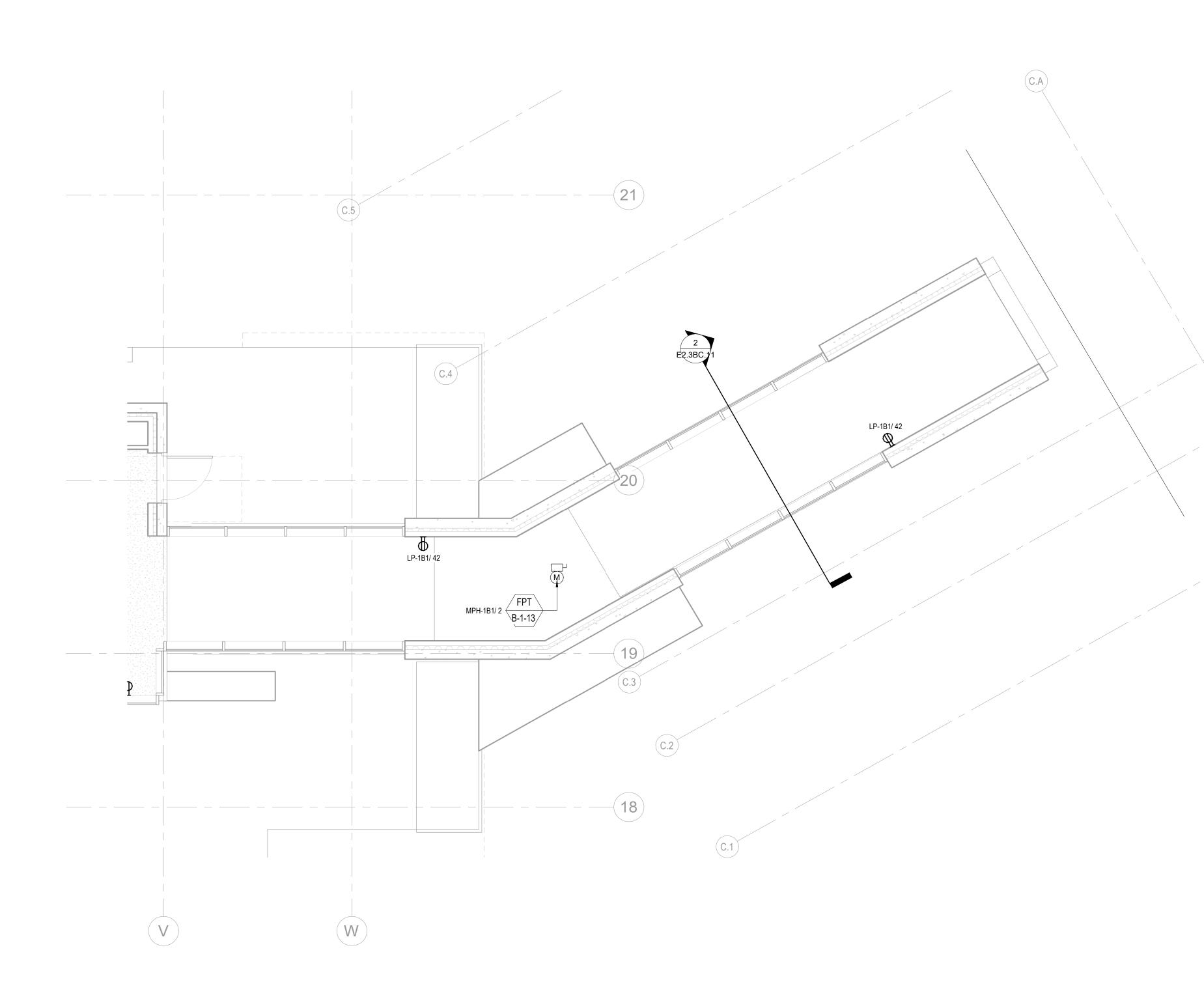
1 TOWER BC - LVL 1 CONNECTOR ELECTRICAL POWER PLAN SCALE: 1/4" = 1'-0"
