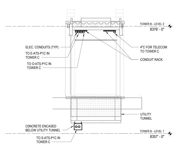
2 TOWER BC - CONNECTOR ELECTRICAL POWER SECTION SCALE: 1/4" = 1'-0"
