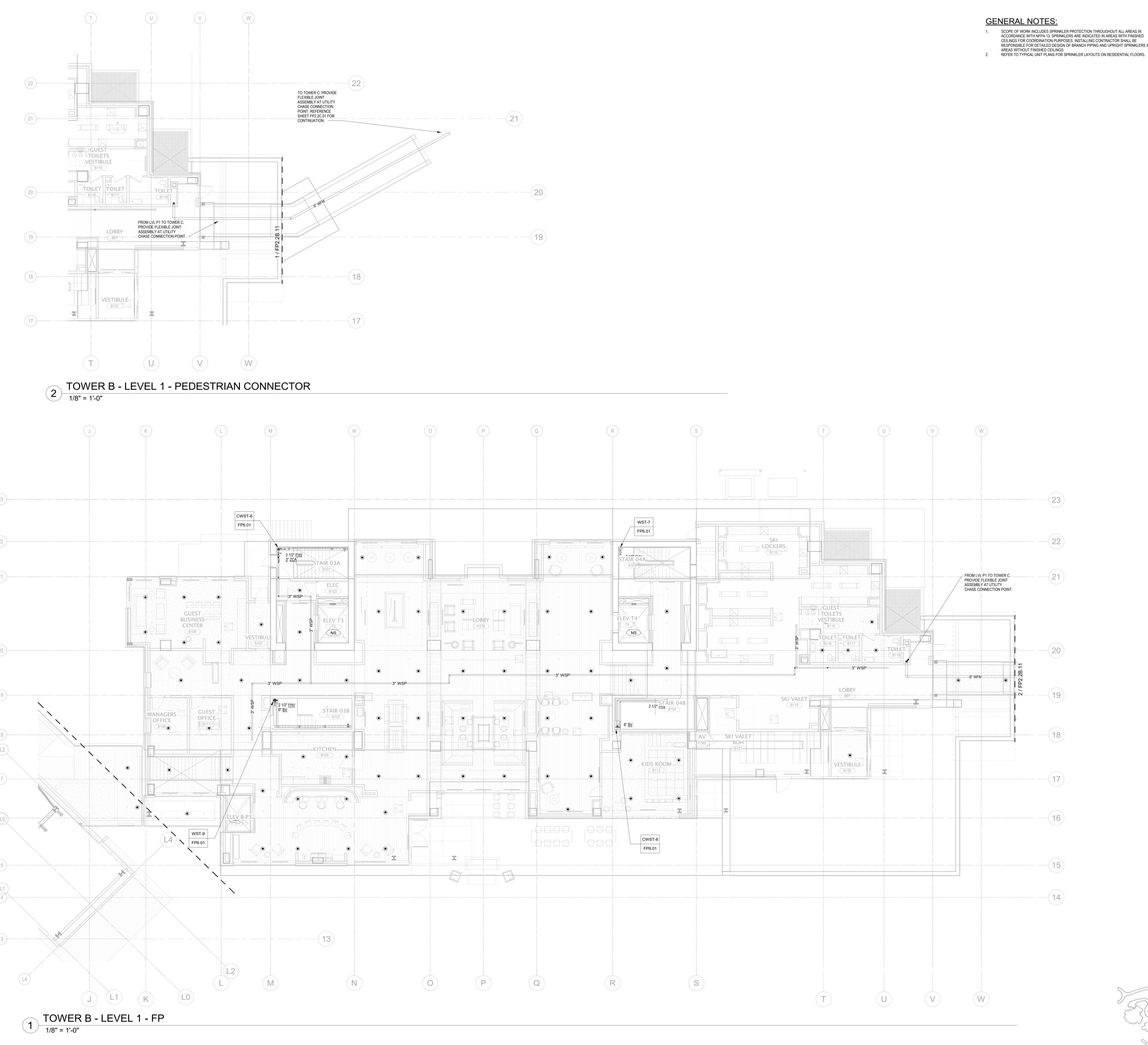
SCOPE OF WORK INCLUDES SPRINKLER PROTECTION THROUGHOUT ALL AREAS IN ACCORDANCE WITH NFPA 13. SPRINKLERS ARE INDICATED IN AREAS WITH FINISHED CEILINGS FOR COORDINATION PURPOSES. INSTALLING CONTRACTOR SHALL BE RESPONSIBLE FOR DETAILED DESIGN OF BRANCH PIPING AND UPRIGHT SPRINKLERS IN
