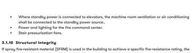
minimum bond strength of the SFRM must be 430 pounds per square foot. **3.1.11 Fire Service Access Elevators**
