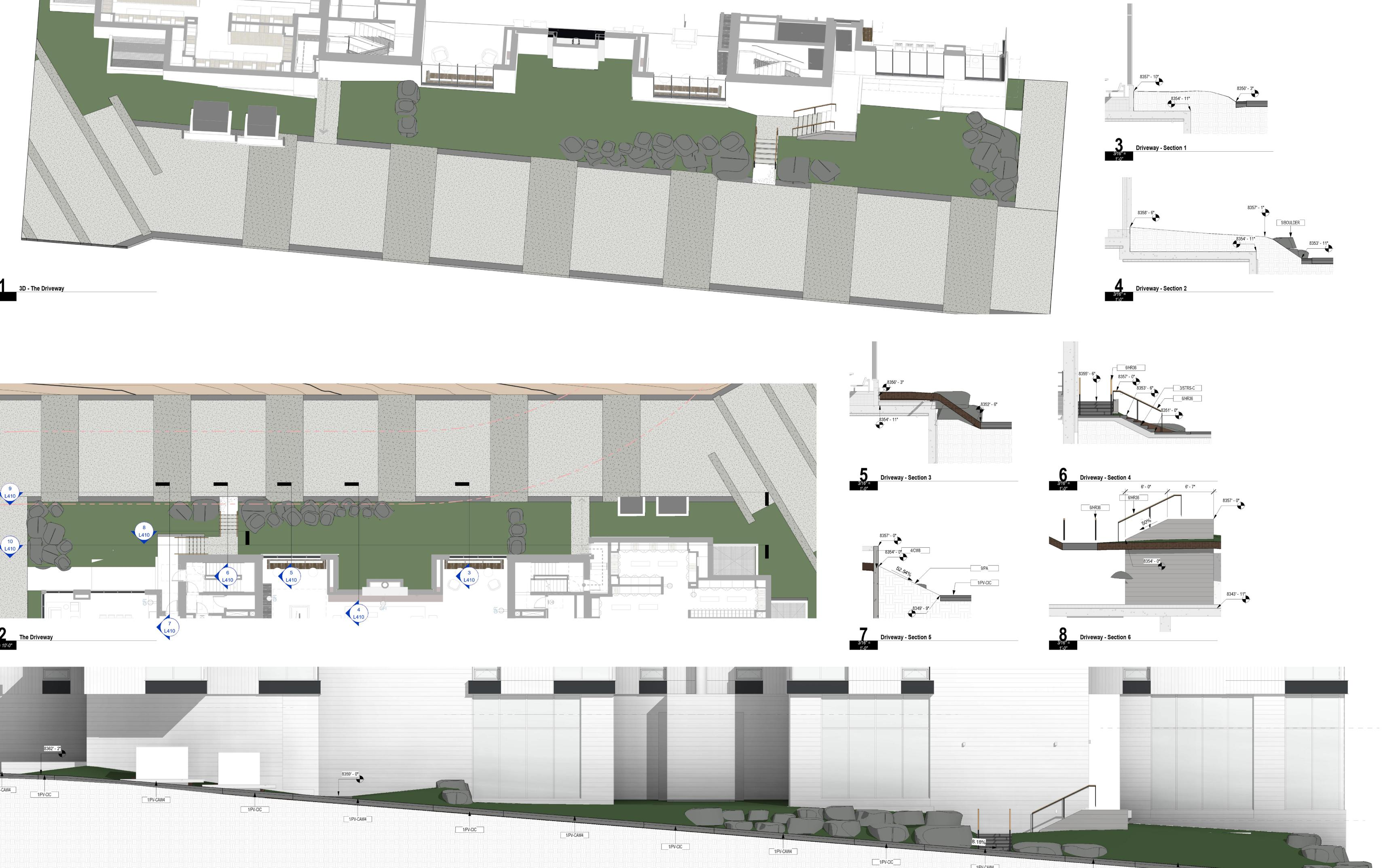
01 PAVEMENT, RAMPS, AND CURBS 4/L401 1,400 SF 6/L401 952 SF Crushed Stone with Agg Base Mexican Pebble with Agg Base 1/PV-C
