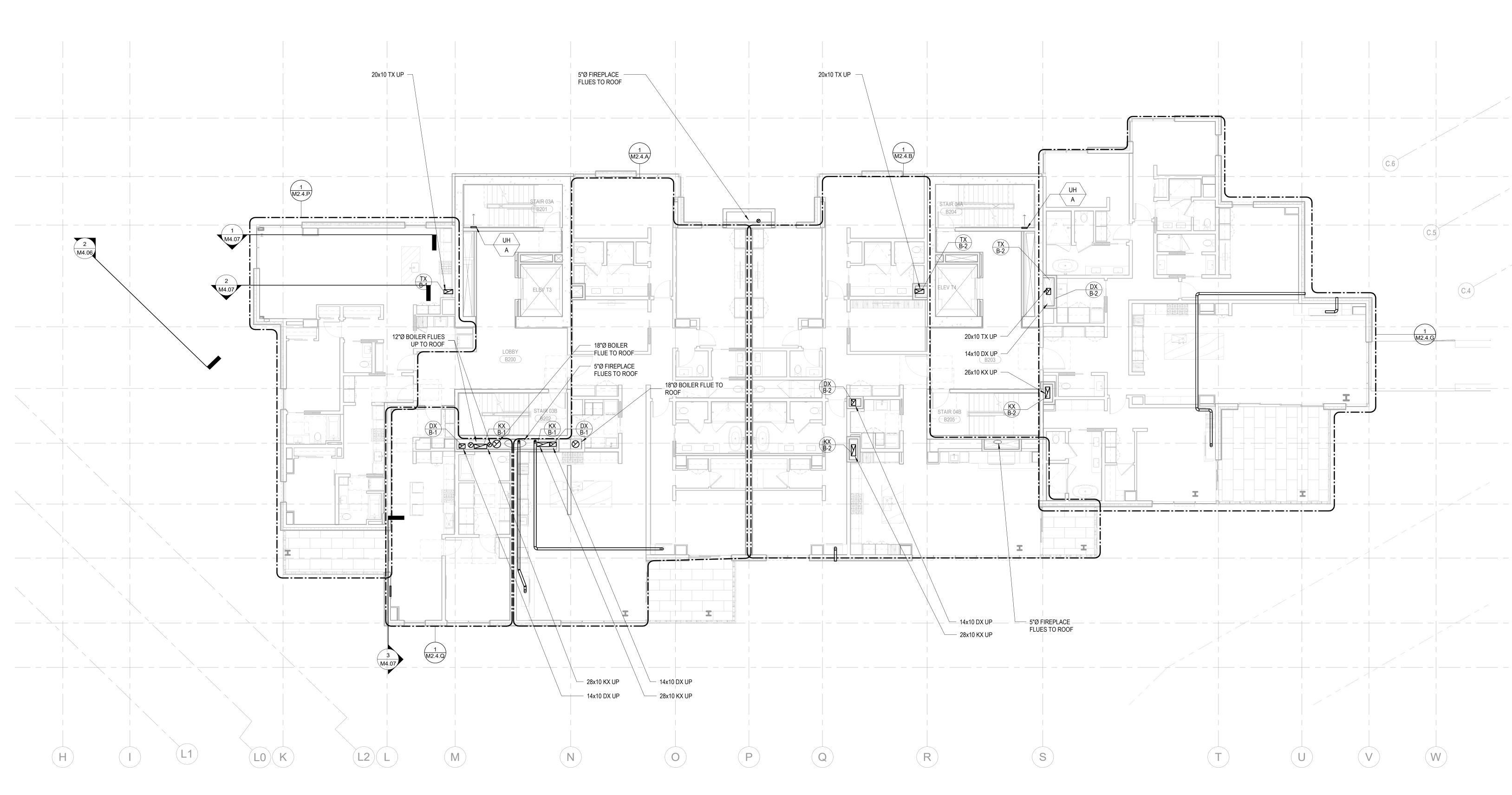
1 TOWER B - LEVEL 2 MECHANICAL DUCT PLAN SCALE: 1/8" = 1'-0"
