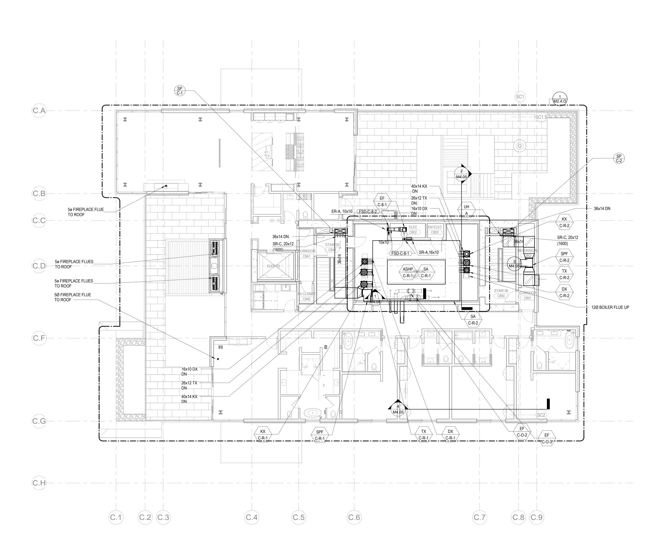
1 TOWER C - LEVEL 8 MECHANICAL DUCT PLAN SCALE: 1/8" = 1'-0"
