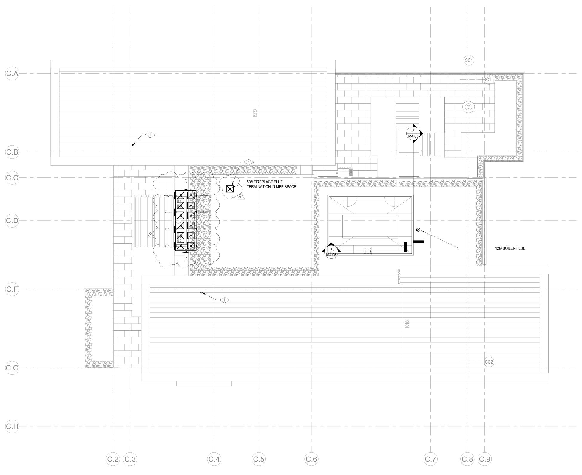
1 TOWER C - ROOF MECHANICAL DUCT PLAN SCALE: 1/8" = 1'-0"
