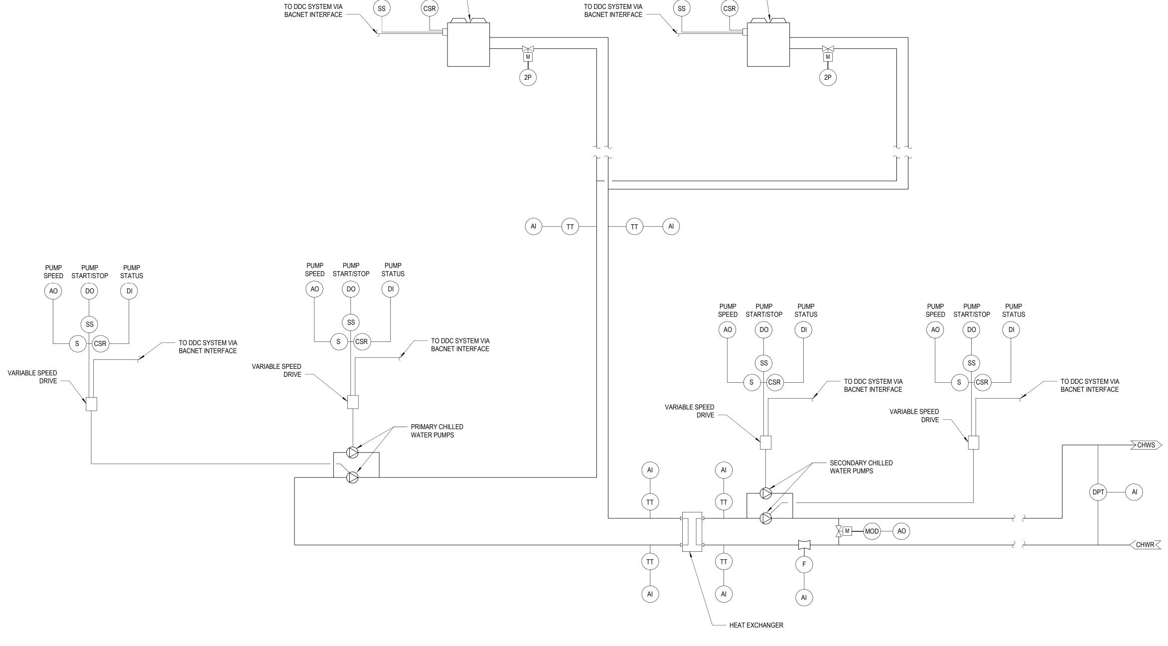
CHILLED WATER SYSTEM CONTROL DIAGRAM - TOWER A&B SCALE: NTS
