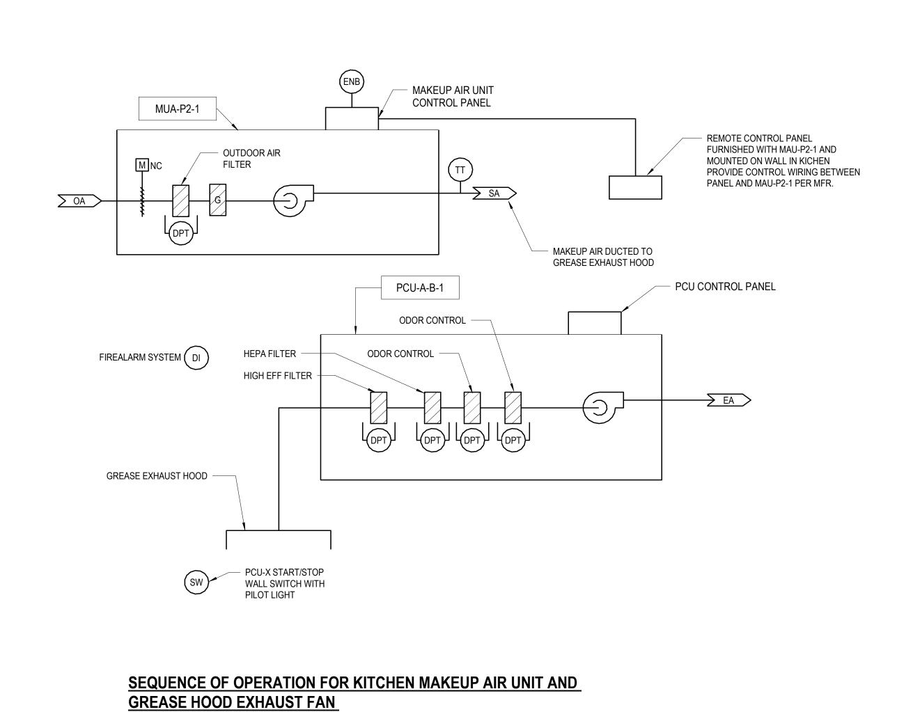
A. THE SYSTEM CONSISTS OF A 100% OUTSIDE AIR MAKEUP AIR UNIT (MAU-P2-1) WITH CONSTANT SPEED SUPPLY FAN,
