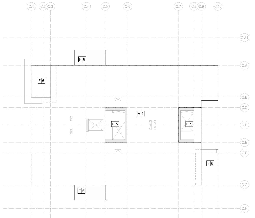
LOAD MAP KEY: NUMBER INDICATES SUPERIMPOSED DEAD LOAD MARK LETTER INDICATES LIVE LOAD MARK INDICATES CLADDING LOAD IN POUNDS PER SQUARE FOOT OF SURFACE AREA.
