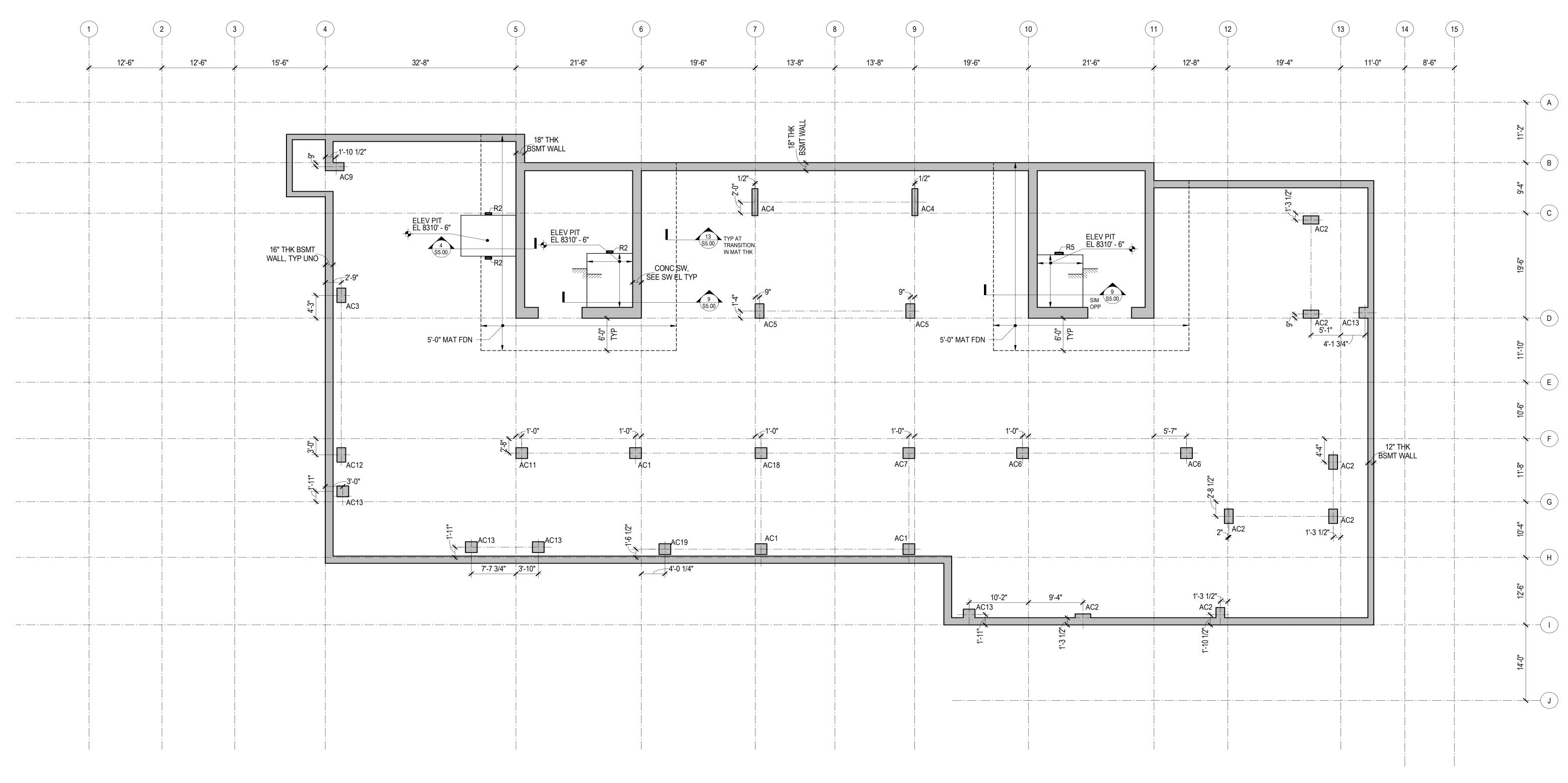
TOWER A - LEVEL B1 FRAMING PLAN
