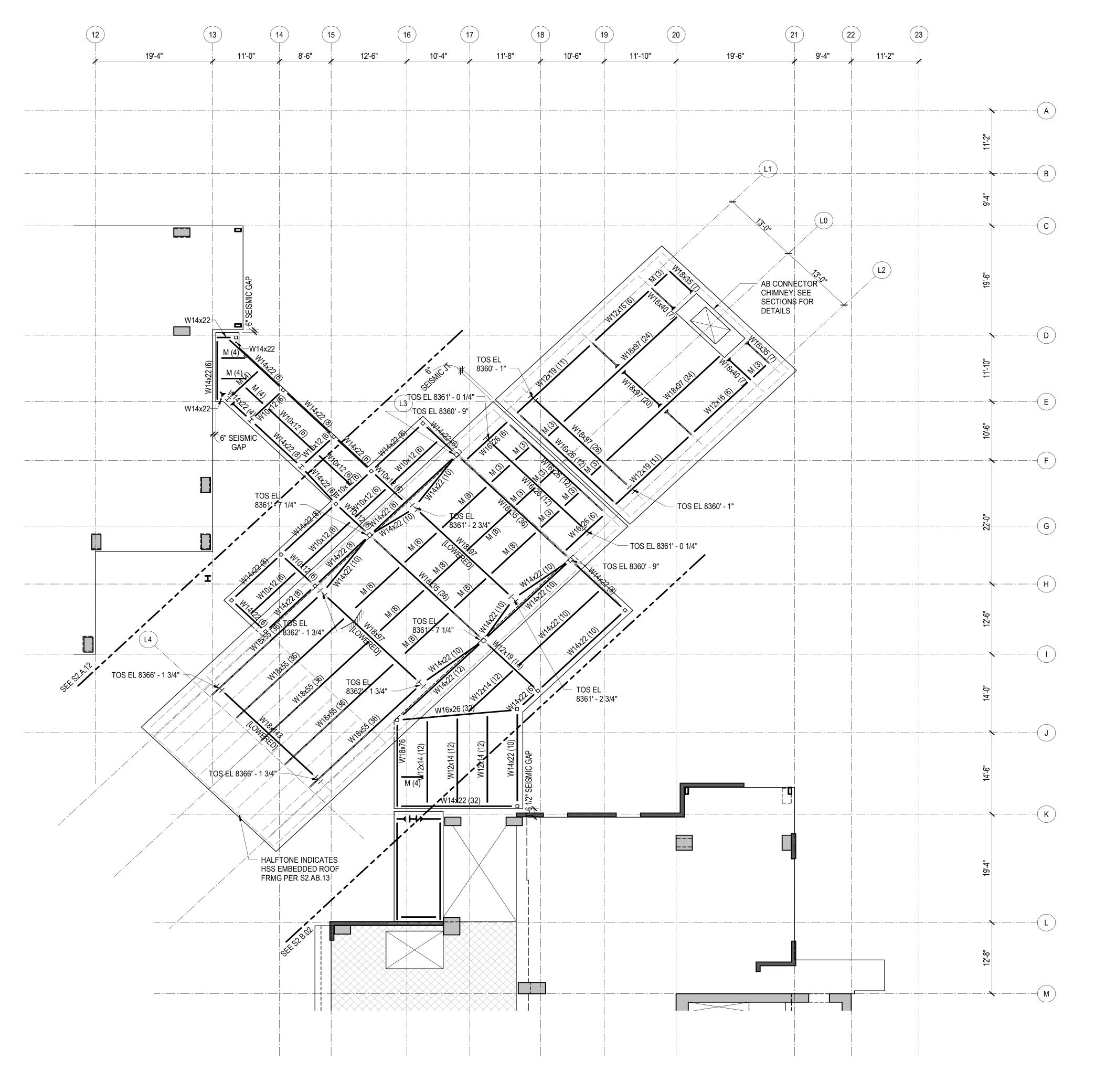
TOWER A & B - ROOF LEVEL FRAMING PLAN
