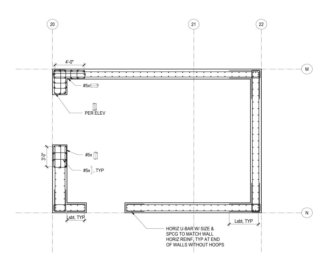
7 SHEAR WALL SECTION - LEVEL 4 TO LEVEL 7
