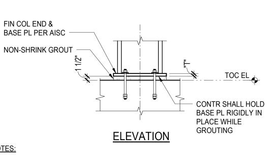
TIGHTEN ANCHOR RODS SNUG TIGHT AND SCORE ROD THREADS TO PREVENT
