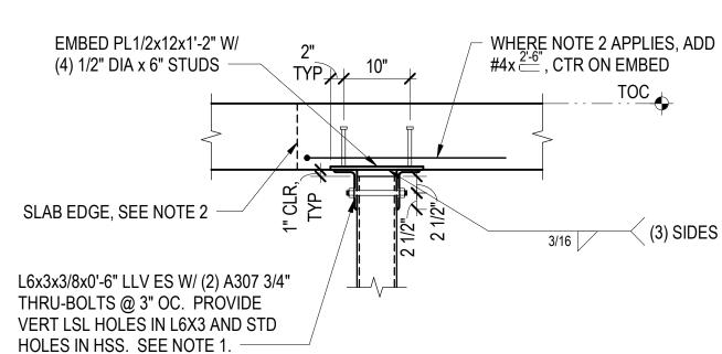
1. WHERE NOTE APPLIES, BOLT TO BE CENTERED IN SLOTTED HOLE IN ANGLE. NUTS TO BE FINGER TIGHT. DAMAGE THREADS OF BOLT TO PREVENT BACK-OFF OF NUT.
