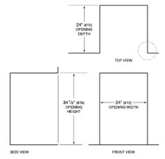
NOTE: 3<sup>1</sup>/2" (89) finished returns will be visible and should be finished to match cabinetry.
