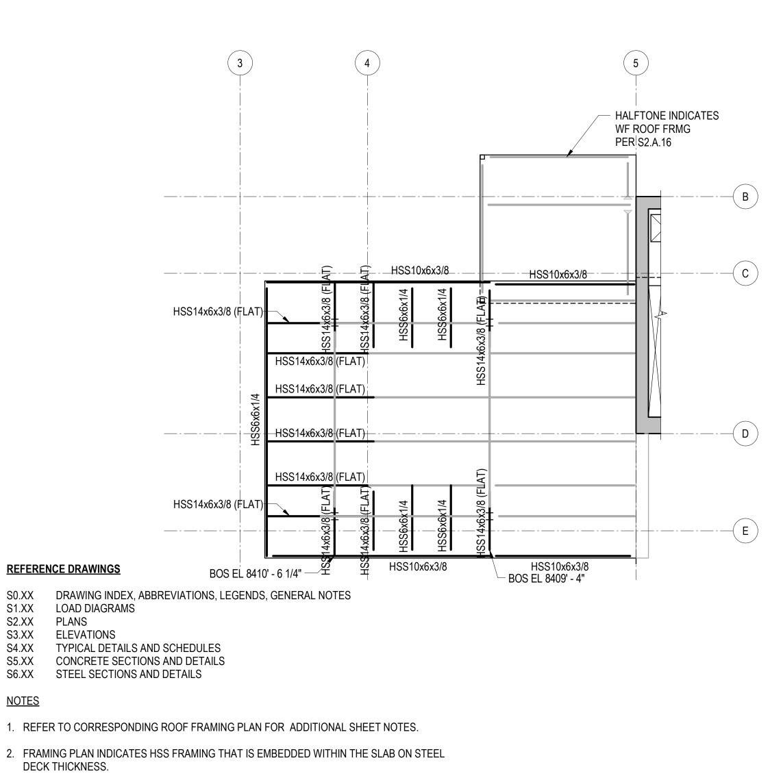
3. BOTTOM OF STEEL IS AT THE BOTTOM OF SLAB ON STEEL DECK. PARTIAL PLAN - LEVEL 6 EMBEDDED HSS ROOF FRAMING THERMAL BREAK AT HSS8x8x5/8-GLASS, TYP (4) LOCS 3" LWC ON 3" STL DECK; TOC AT TOP OF BM HSS12x8x5/8 (FLAT) H\$S10x8x3/8 (FLAT) HSS8x8x3/8 W14x90 [-1/2"] [-1/2"] HSS10x8x3/8 (FLAT), TYP′≌
