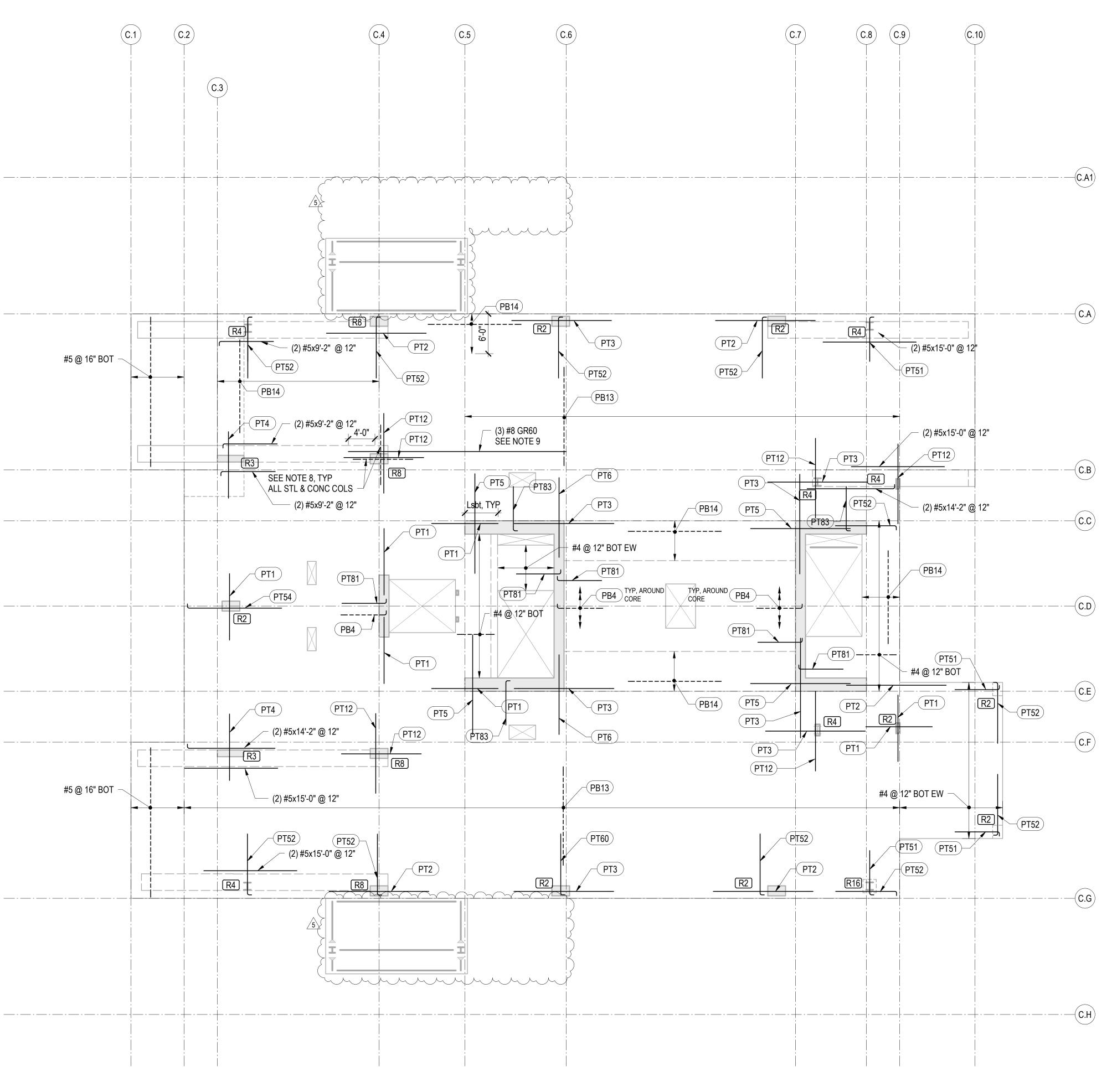
9. WHERE NOTE APPLIES, REINFORCEMENT IS TO BE PLACED WITHIN VERTICALS OF COLUMN NEAR GRID C.4/C.B. REINFORCEMENT SHALL BE CENTERED IN SLAB MID-DEPTH. REINFORCEMENT SHALL MEET CENTER-TO-CENTER SPACING OF 3db BUT NOT LESS THAN 3-INCHES, UNLESS NOTED OTHERWISE. LAP SPLICE IS NOT PERMITTED; PROVIDE MECHANICAL COUPLER IF NECESSARY.
