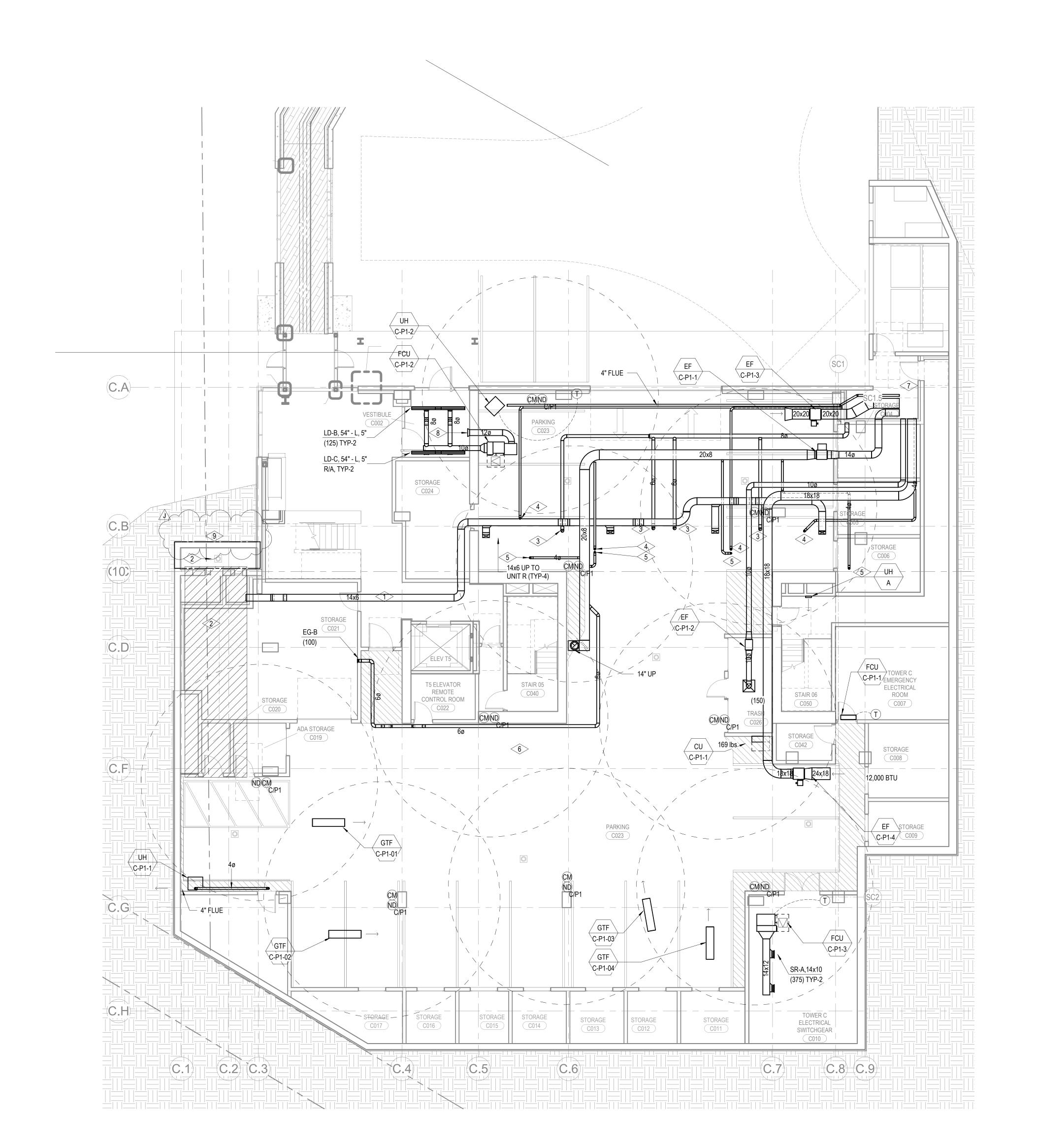
1 TOWER C - PARKING LEVEL MECHANICAL DUCT PLAN
