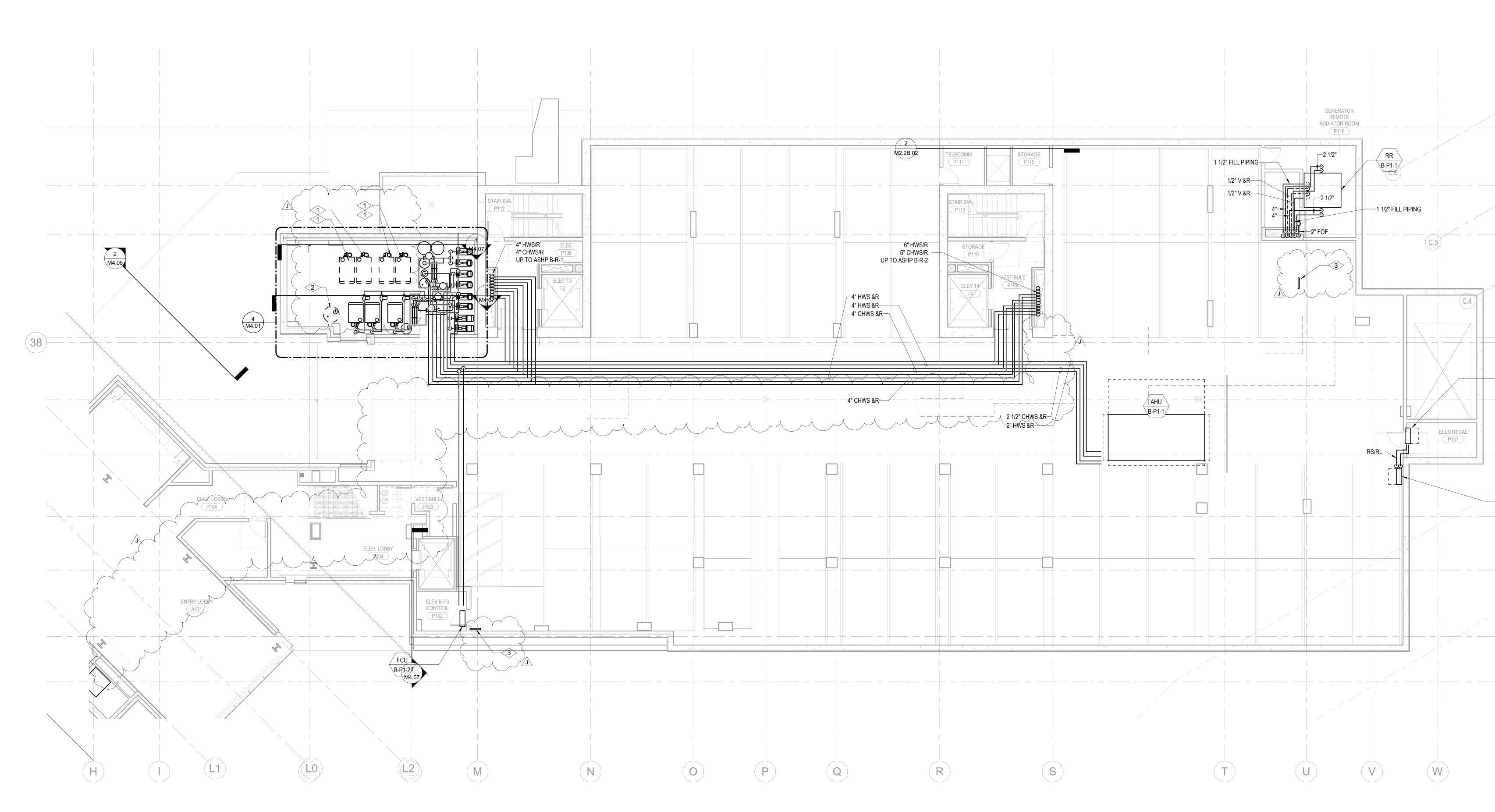
1 TOWER B - PARKING LEVEL 1 MECHANICAL PIPING PLAN SCALE: 1/8" = 1'-0"
