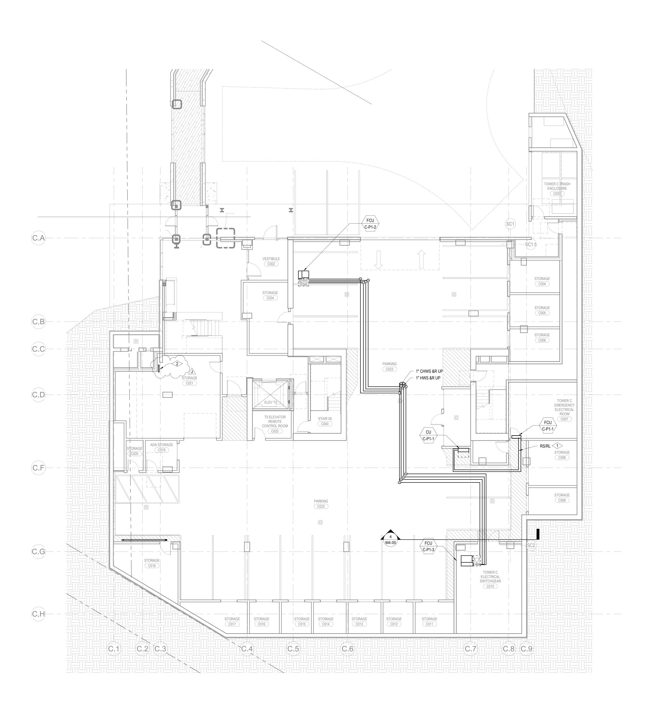
TOWER C - PARKING LEVEL MECHANICAL PIPING PLAN
