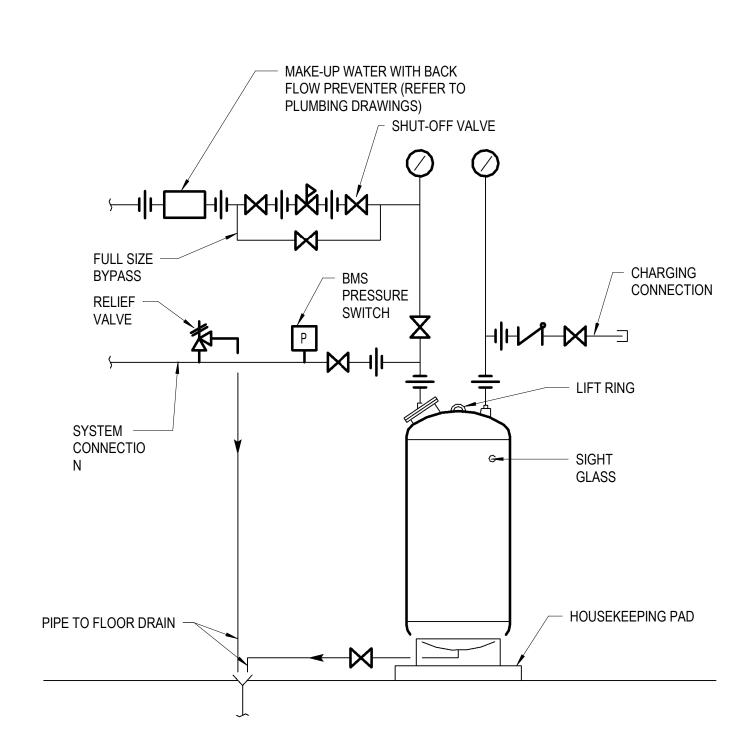
VERTICAL EXPANSION TANK 5 VERTICE SCALE: NTS
