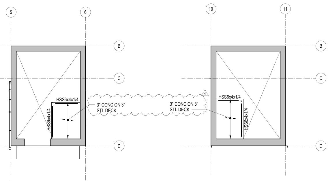
NOTED OTHERWISE. 2. STRUCTURAL SLAB IS 3-INCHES OF CONCRETE ON 3-INCH COMPOSITE STEEL DECK UNLESS NOTED OTHERWISE. REINFORCE WITH WWR 6x6-W2.9xW2.9. SEE TYPICAL SLAB ON STEEL DECK DETAILS FOR REINFORCING AND OTHER INFORMATION. REINFORCING SHOWN ON THE PLAN AND IN THE TYPICAL DETAILS IS IN ADDITION TO THIS REINFORCING.
