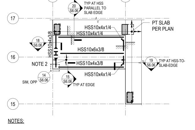
1. SEE RELEVANT PLANS FOR REFERENCE ELEVATION. TOP OF STEEL IS AT BOTTOM OF DECK UNLESS NOTED OTHERWISE
