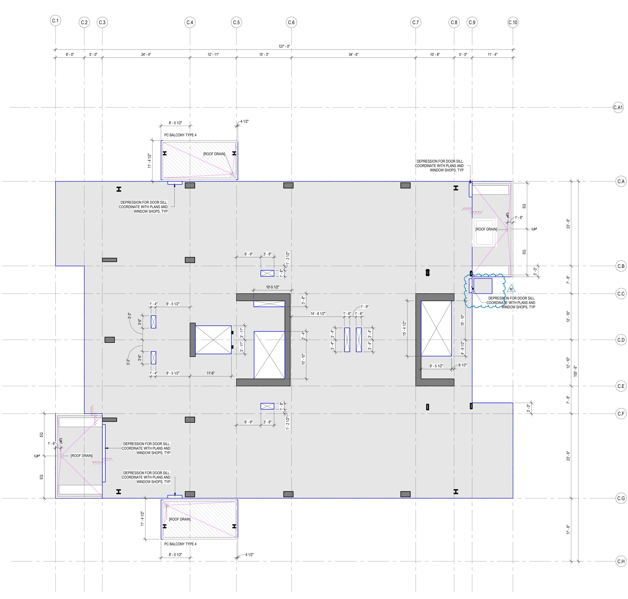
1 CONCRETE PLAN - TOWER C - LVL 4 SCALE: 1/8" = 1'-0"
