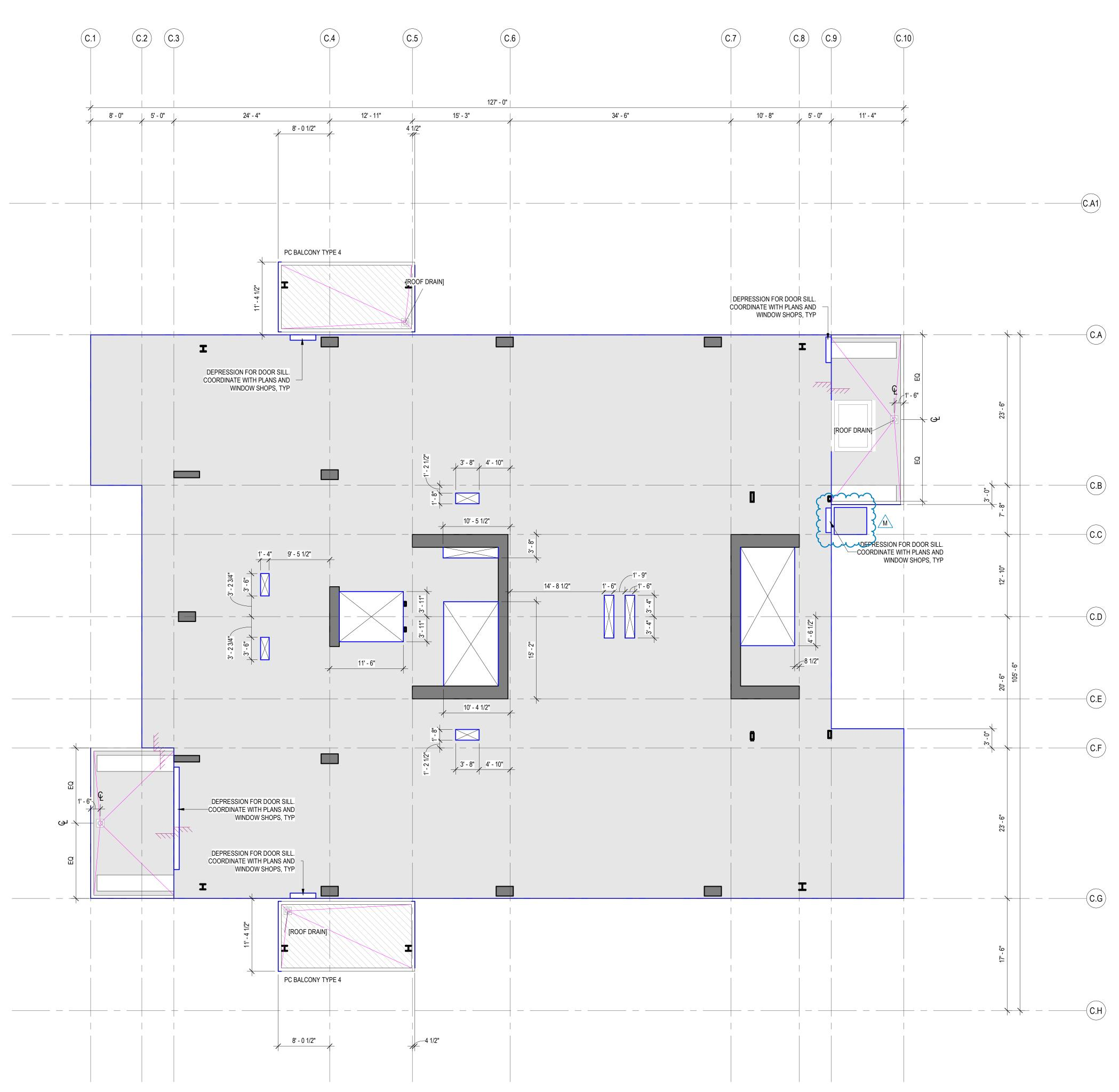
1 CONCRETE PLAN - TOWER C - LVL 6 SCALE: 1/8" = 1'-0"
