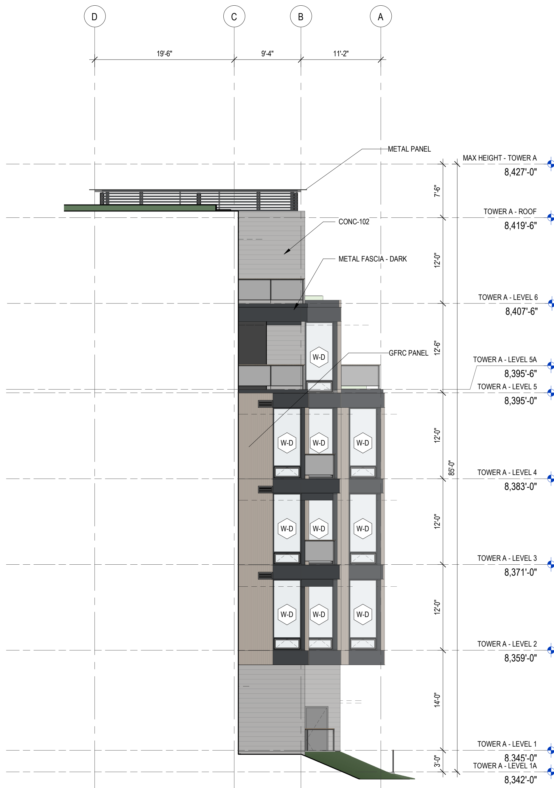
6 TOWER A - PARTIAL WEST SCALE: 1/8" = 1'-0"
