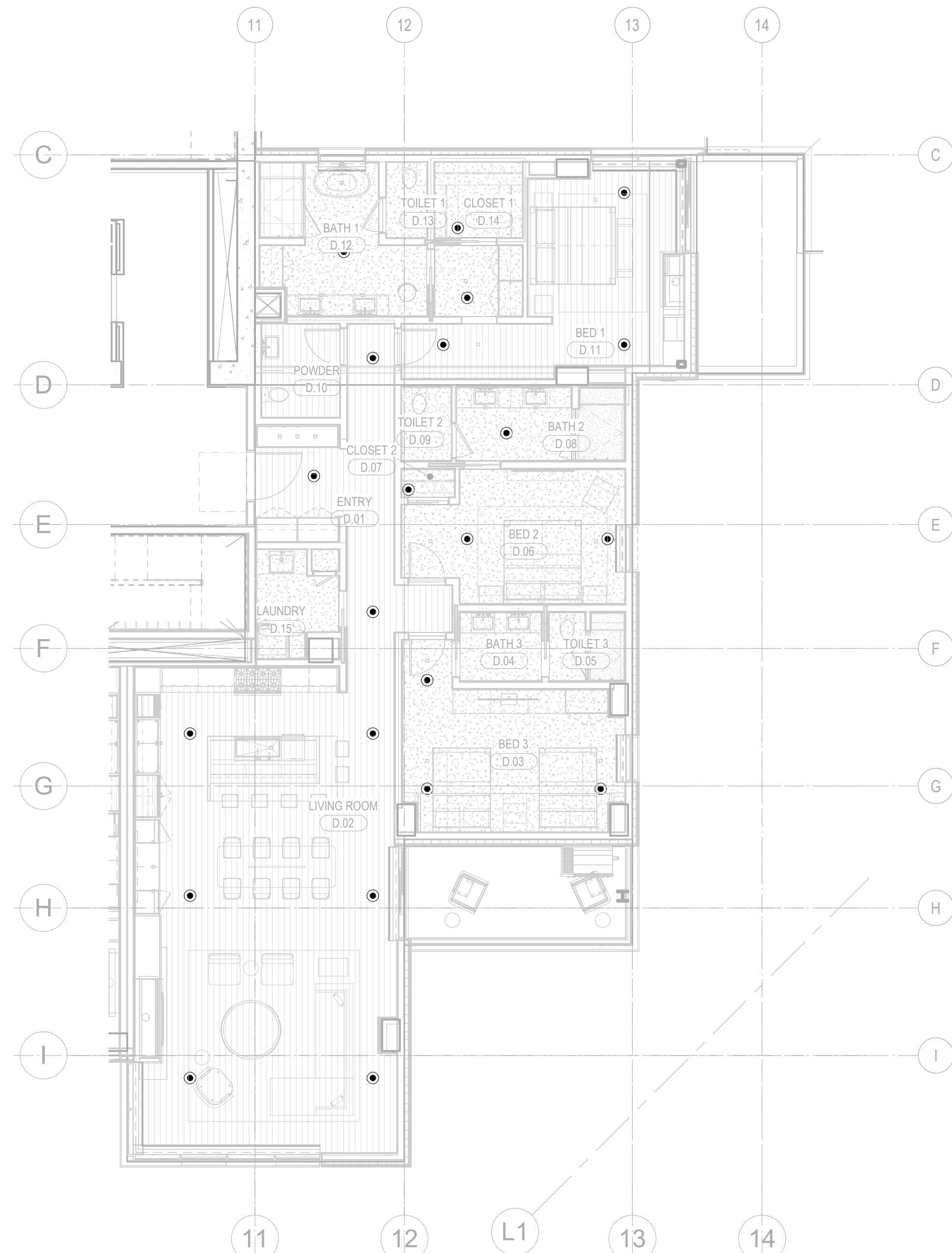
4 ENLARGED PLAN - TOWER A/B-UNIT D 1/8" = 1'-0"
